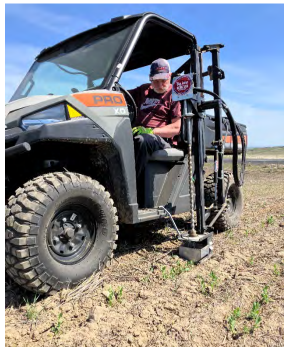
Above: Soil sampling at JS-14 using a UTV-mounted automated auger sampler. Also note low cover crop biomass coming out of winter.
